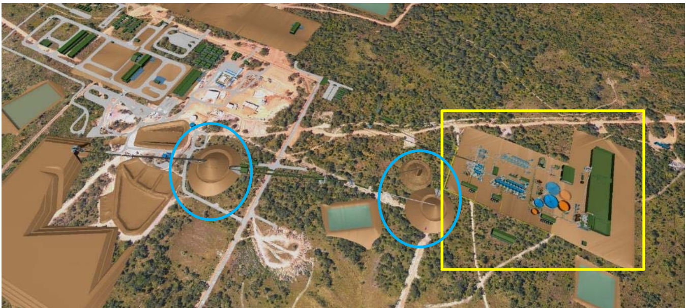
Figure 4: Kakula’s conceptual surface layout, showing the ore stockpiles (blue circles) and processing plant (yellow box).
